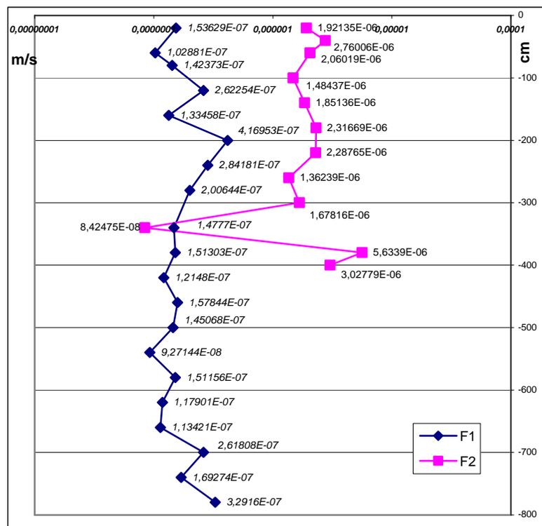
Fig. 2. The „k” infiltration velocity at different depth.
