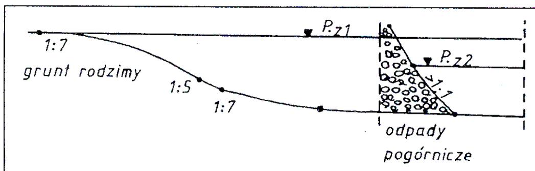
Fig. 1. The changes in transverse profile in the zone of filling up of water reservoir
