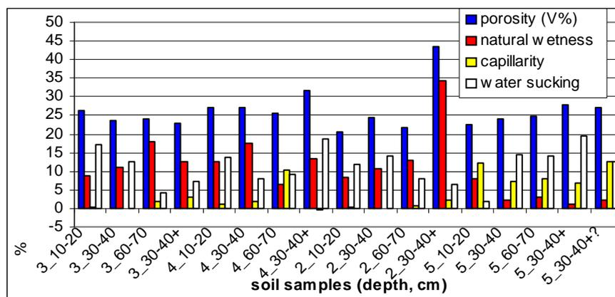
Fig 5. The hidrologic parameters of soil samples from the heap
