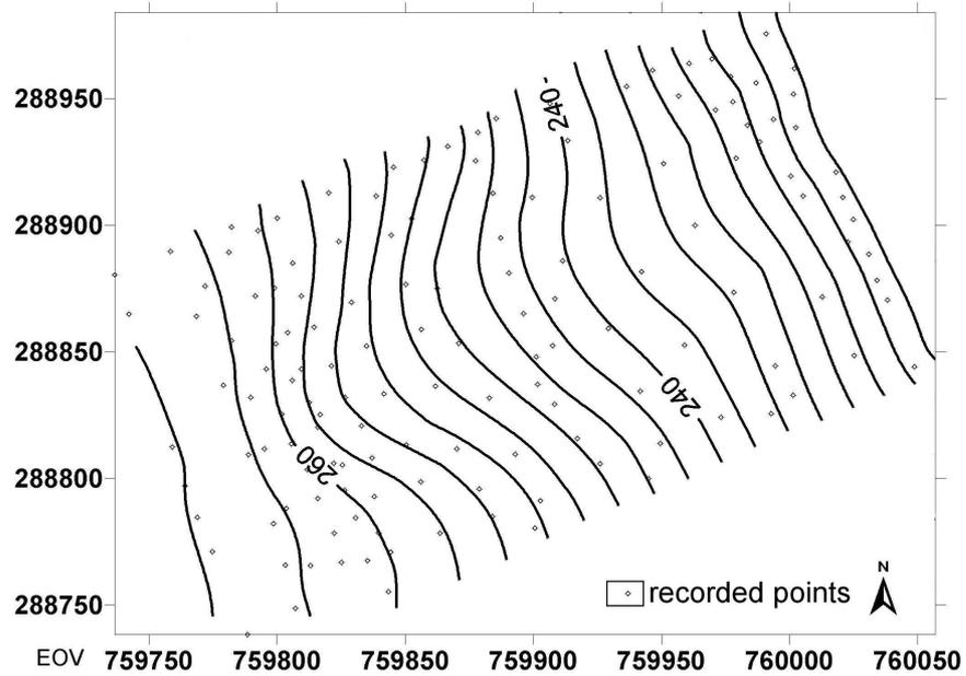
Fig. 2. Distribution of the survey points in the sample area with the elevation contour lines
