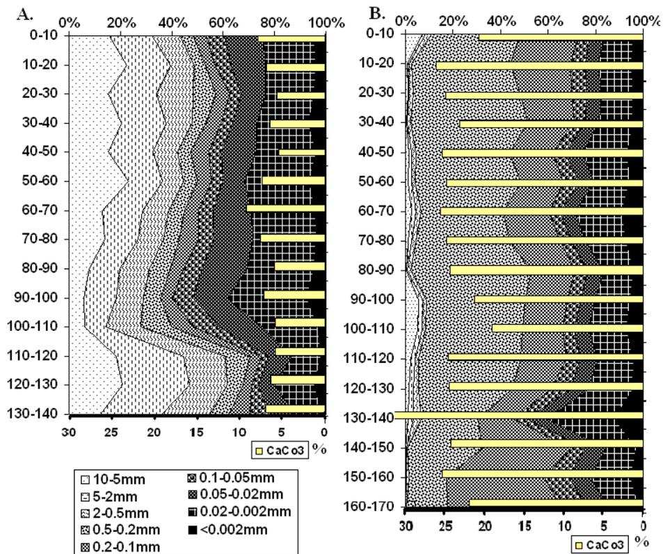
Fig. 3. Particle size distribution and CaCO<sub>3</sub> contents behind the destroyed dry stone walls on the Sátor Hill (A.) and the Csobánc Hill (B.)
