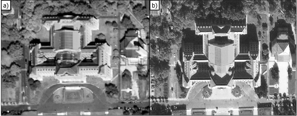
Figure 2. Differences in perspective due to different off-nadir angles of (a) WorldView-2 and (b) WorldView-3 in the example of the main building of the University of Debrecen
